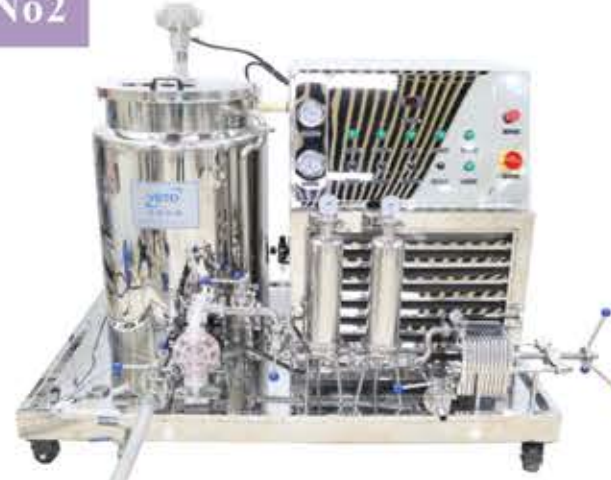
Perfume making machine with two filters
